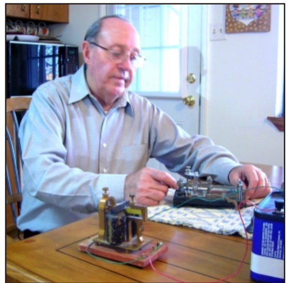
Photo: Paul Harden Roy Carrejo sends morse code on his Vibroplex speed-key and sounder — still in working condition.
